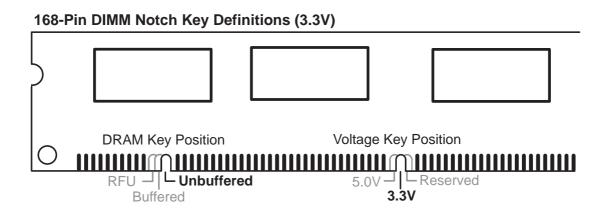
The notch on the DIMM module will shift between left, center, or right to identify the type and also to prevent the wrong type of DIMM to be inserted into the DIMM socket on the motherboard. Four clock signals are supported on this motherboard. You must ask your retailer for the specifications before purchasing memory modules.
