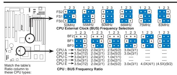
Set the jumpers by the Internal speed of the Intel, AMD, IBM, or Cyrix CPU as follows:
