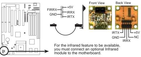
Infrared Module Connector
