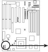
**TIP:** If the case-mounted LED does not light, try reversing the 2-Pin plug.
