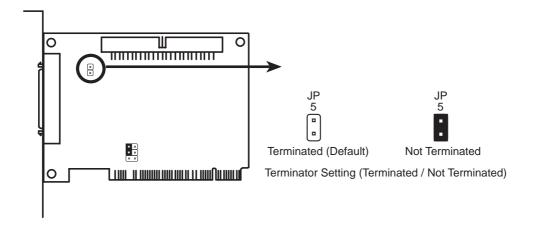
Decide whether or not you need to terminate the ASUS PCI-SC200 based on its position in the SCSI chain. Only the devices at each end of the chain need to be terminated. If you have **only** internal or **only** external devices connected to the ASUS PCI-SC200, then you **must** terminate the ASUS PCI-SC200. If you have **both** internal and external devices connected, you **must not** terminate the card. See the following example which illustrates this concept.
