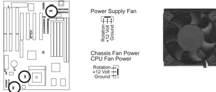
12Volt Chassis, CPU, Power Supply Fan Power
