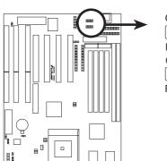
COM 1 ••••• Pin 1 COM 2 ••••• ••••• Pin 1 For these connectors to be available, you must connect the included Serial cable set from COM1 (using the 9-Pin male) & COM2 (using the 25-Pin male) to a free expansion slot opening.
