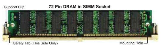
To release the memory module, push both support clips outward and rock the module out of the support clips.
