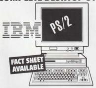
120Mb hard drive, 4Mb RAM, 1Mb video, 16K cache, 1.44Mb floppy, choice of PCMCIA or single 16 bit ISA slot. IBM keyboard with TrackPoint pointing device, 14" mono VGA, DOS/Win 3.1.
