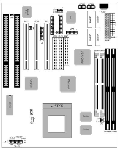
Figure **2-1**. Mainboard Component Locations
