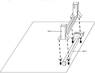
If the retention clip is installed incorrectly, you will not be able to insert the retention clip into the CPU and in this situation you might need to rotate the retention clip by  $180^{\circ}$ .
