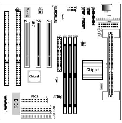
Figure 2-1. Mainboard Component Locations
